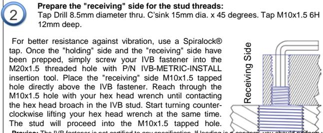
Tighten until the stud is fully engaged (approximately 12mm into the "receiving" side). Use a feeler gauge to insure that the "receiving" side material is pulled down properly.
